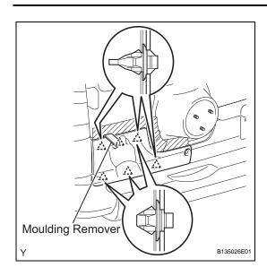
(c) Using a moulding remover, disengage the 6 clips and remove the back door outside moulding.
