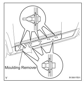
(c) Using a moulding remover, disengage the 9 clips and remove the front door outside moulding.
