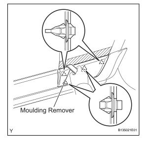
(c) Using a moulding remover, disengage the 4 clips and remove the access door outside moulding.
