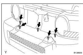
(c) Remove the 8 screws and the 4 bolts.
