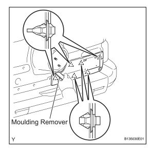
(c) Using a moulding remover, disengage the 6 clips and remove the back door outside moulding.
